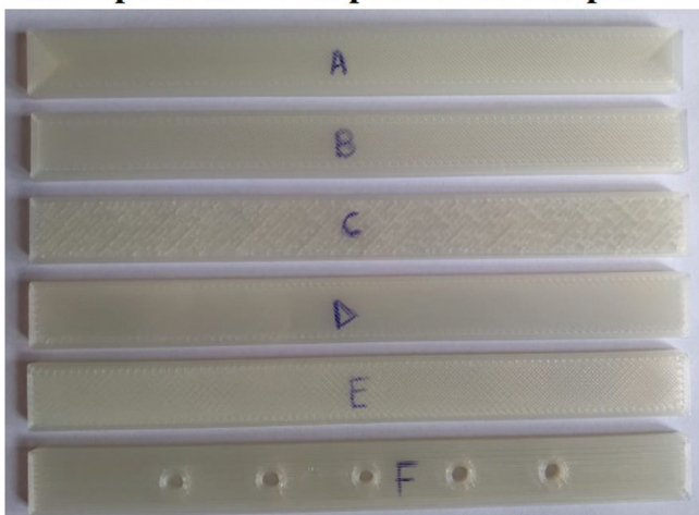
Figure 2. PLA printed samples with different infill patterns.
